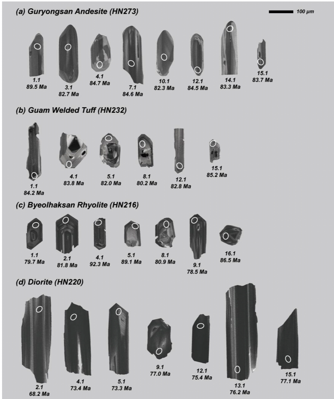
Fig. 2. Representative Cathodoluminescence images of the analysed zircon grains, showing the location of analytical spots and ^{206}\text{Pb}/^{238}\text{U} ages in Ma, separated from the Guryongsan Andesite (HN273), Guam Welded Tuff (HN232), Byeolhaksan Rhyolite (HN216) and Diorite dyke (HN220).
