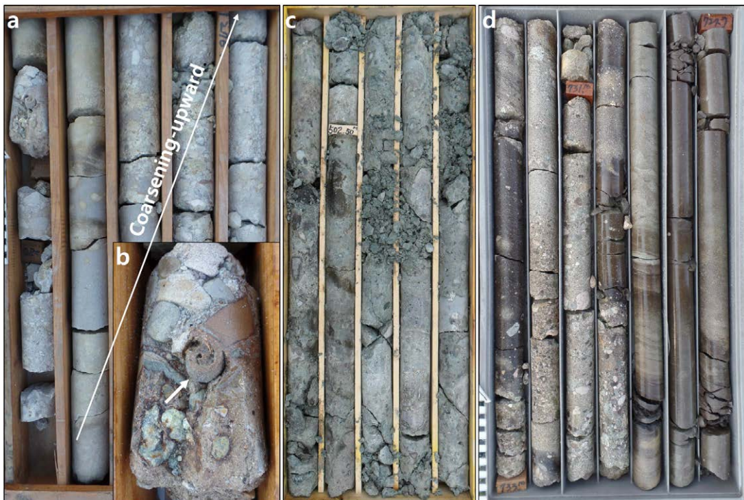
Fig. 14. (a) Coarsening-upward trend of muddy sandstone and breccia, just above the basement (Paleocene to Eocene lapilli tuff) of H-well. (b) Gastropoda fossil in the lowest part of H-well, (c) Breccia in the lowest part of PH-CLH-2 well. Previous studies interpreted this interval as Cretaceous basement (KIGAM, 2014). However, intercalating muddy sandstone and mud matrix in the breccia suggest that this interval was deposited during the Miocene. (d) Cretaceous conglomerate, sandstone and mudstone around 730 m interval of B-well. Previous studies interpreted this interval as a Yeonil Group (Han et al. , 1986). However, brownish mudstone and rounded clasts as well as locally lithified units suggest that this interval is a Cretaceous sedimentary rock.
