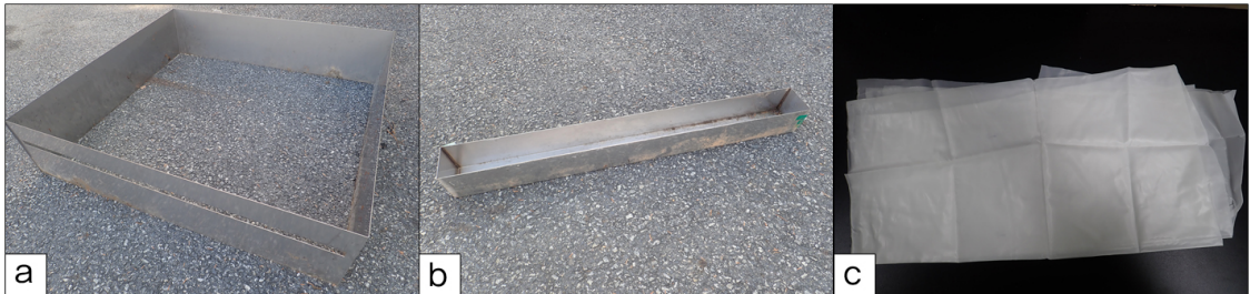
Fig. 11. Equipments for mountain slope sediment trap. a: Metal plot, b: sediment trap, and c: 10 µm mesh-size nylon sieve for sediment collecting.
