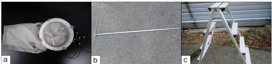
Fig. 9. Equipments for anemophilous (wind-driven) pollen trap. a: Trap, b: T-shaped trap holder, c: Ladder used to retrieve pollen trap.
