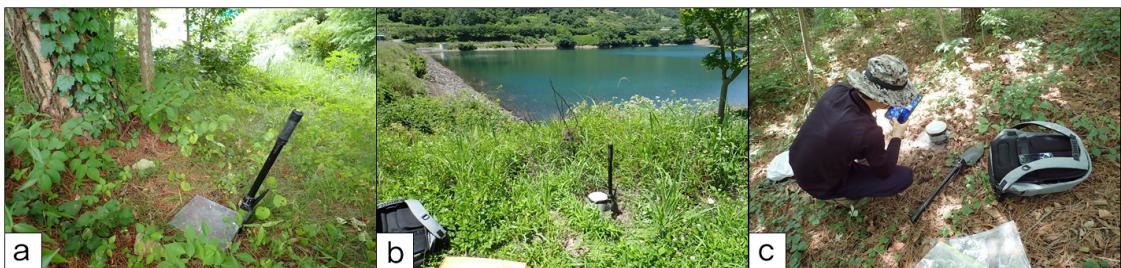
Fig. 13. Equipments for collecting surface soil samples. a: Sampler, b and c: Sampling location acquisition using Global Positioning System (Model: Trimble R2).
