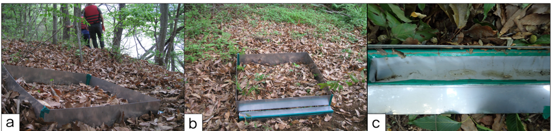
Fig. 12. Installing and collecting process of mountain slope sediment trap. a and b: Install a plot, and c: Retrieving the pollen and sediments.
