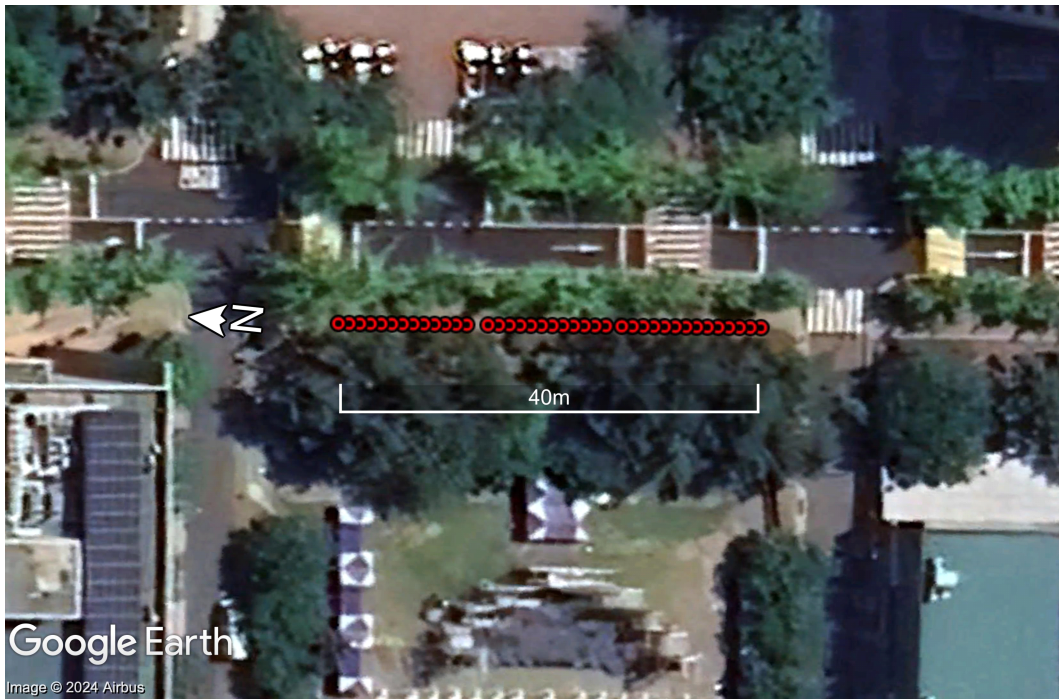
Fig. 9. Deployment of a geophone array for the field experiment. An aerial view shows the linear arrangement of geophones denoted with red dots spanning about 40 m along a roadway for traffic-induced seismic noise monitoring.
