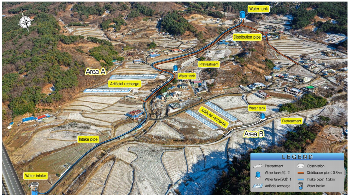
Fig. 7. Landscape of Hybrid-type artificial recharge and circulation system in the study area.
