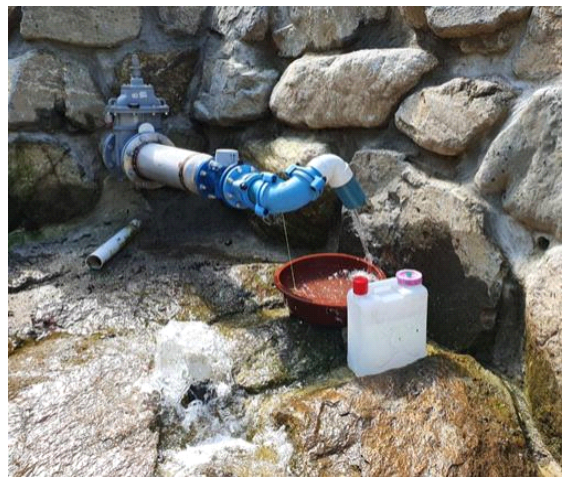
(d) Sand dam outflow rate measurement using flow meter
