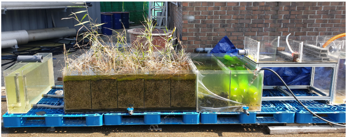
Fig. 4. Pre-treatment system of stream water.
