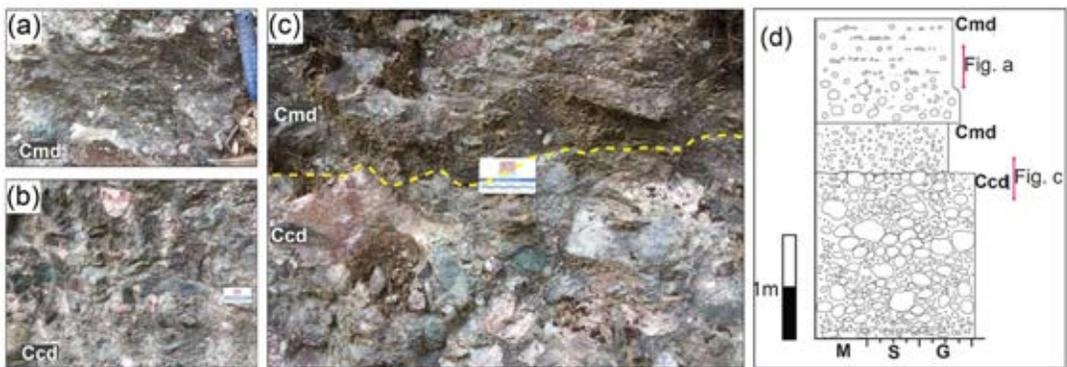
**Fig. 6.** Photographs and columnar log of Facies Association II. (a) Matrix-supported, disorganized conglomerate. (b) Clast-supported, disorganized conglomerate showing poor sorting and sub-rounded to rounded roundness. (c) Irregular contacts between clast-supported, disorganized conglomerate and matrix-supported, disorganized conglomerate. (d) Sketched columnar log of Facies Association II (Cmd: Matrix-supported, disorganized conglomerate, Ccd: Clast-supported, disorganized conglomerate).
