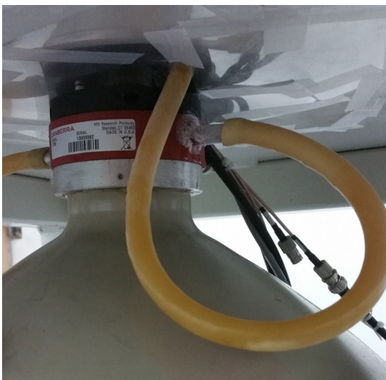
Fig. 6. \text{N}_2 gas purging by liquid nitrogen to eliminate moisture.
