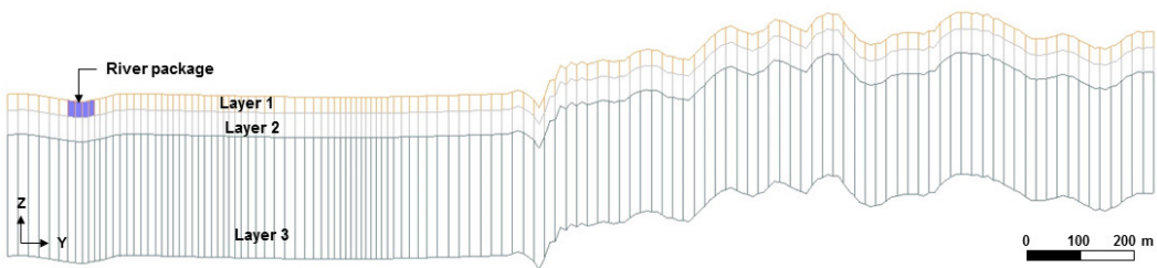
Fig. 3. Cross-section of the constructed aquifer model.
