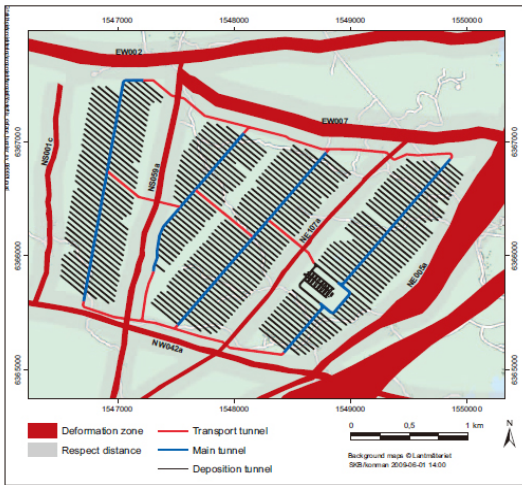
Fig. 4. Layout of a disposal system considering a respect distance from a fault (SKB, 2011).
