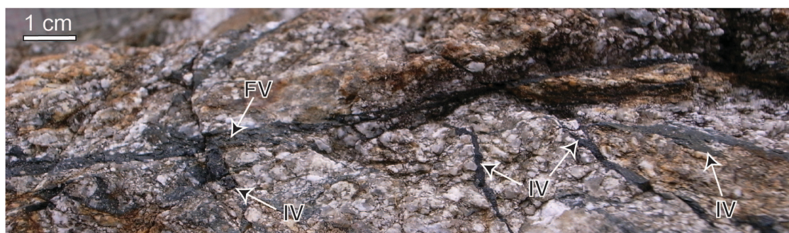
Fig. 1. Outcrop photograph of blackish pseudotachylite in granitic gneiss, Oshima Island, Yawatahama, Japan. Fault vein (FV) of the pseudotachylite is developed along the slip surface and is associated with several injection veins (IV) into the wall rock.
