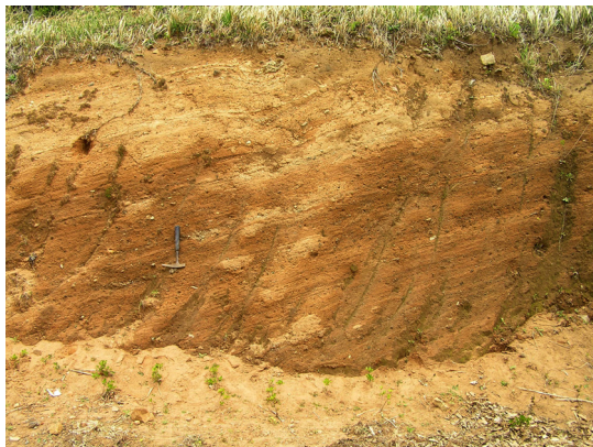
Fig. 7. Hyperconcentrated flow sandstone of the Tamna Formation. Site: 3 on Road 1136 in Tosan-ri. Altitude: about 70 m. Photograph by Sun Yoon on April 29, 2005.
